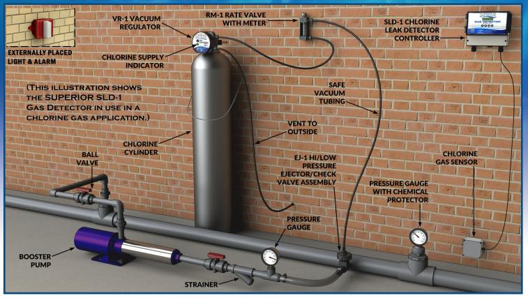
The unit can be placed where it is most convenient for the operator, up to 1,000 feet (305 meters) away from sensors in a monitored environment. Now available with optional, extended life, 3000mAh battery backup.
