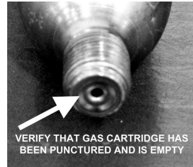
FIGURE 4.2.7 – GAS CARTRIDGE end cap punctured
