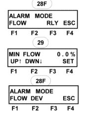
5.4.3.2 **DEV (F2)** opens the Residual Deviation "RES DEV" Menu [30], in the Residual Control and Compound Loop Control Modes. You can set the amount of deviation from the Residual Set Point, in Parts per Million (PPM or mg/L), at which you wish the alarm relay to activate by pressing the UP (F1) or DOWN (F2) keys.
