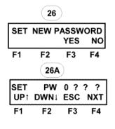
5.1.5.2 After the last digit is entered, pressing the ENT key (F4) shows the "NEW PASSWORD STORED" menu [26B, or 33], and then automatically exits to the Main Menu [1].
